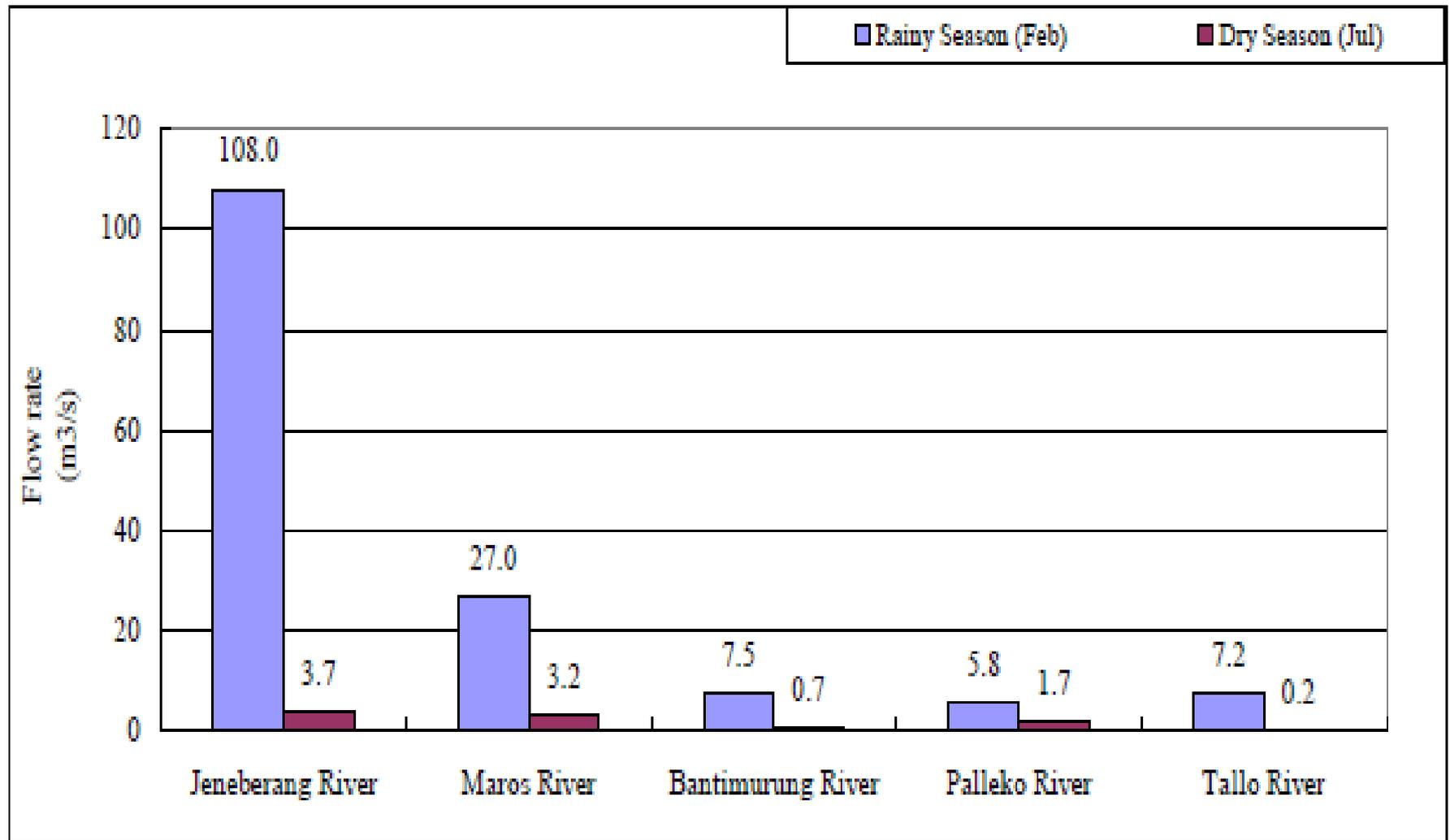
Figure S3.1-1 The results of Flow rate survey
